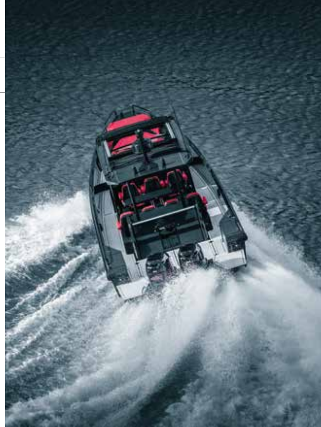
DRY RIDE No matter the speed or conditions, the Brabus Shadow keeps waves out, thanks to a low-set cockpit and plenty of freeboard
